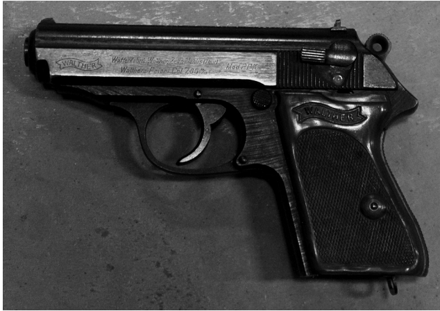
Figure 4.51 A Walther PPK manufactured during World War II. Both the slide and frame are serial numbered and match one another. The finish imperfections and presence of milling marks clearly identify this example as a wartime piece and are common features of wartime German firearms, especially during later stages of the conflict. (Image from author's collection.)
